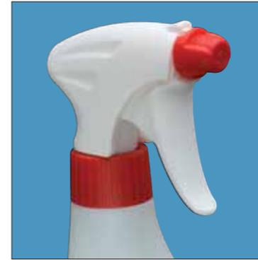
The VELA CR is a child-resistant version of our Vela model, designed for spraying hazardous or aggressive products where child-safety is desired. To begin spraying, a safety button must be pressed and the nozzle turned at the same time. The lock cap fits the sprayer securely to bottles with ratchet finish necks. The Vela CR is ideal for applications such as insecticides, plant care, and acid or alkaline based cleaning products.
